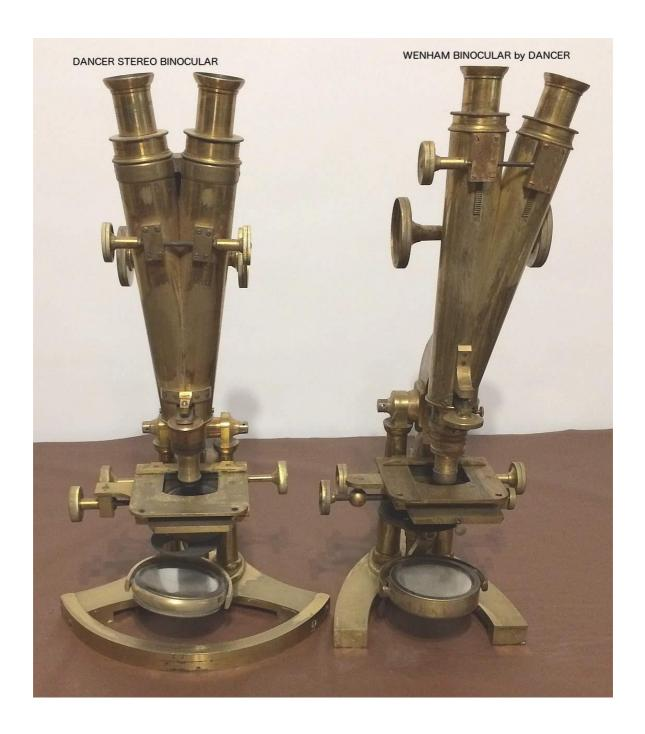
This particular microscope came to me without case or accessories. It is a large stand at about 18 inches high in use, with the Dancer signature on the heel of the foot.
