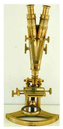
Other attempts were made, including a three part (achromatic?) prism assembly by Dancer. The Dancer method utilised two body tubes in a true "V" format, to split the light into two equal halves, so that each eyepiece receives the same amount of light from the objective. This gives a technically better (albeit more expensive) solution. The Dancer binocular prism method was registered No 4380 June 27th 1861. Compare this with the Wenham prism here.
