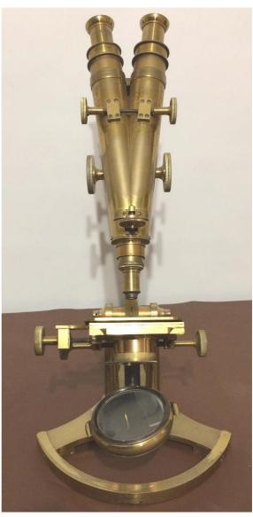
This form of Dancer binocular (stereo) microscope is very rare. I know of only 3 others in captivity and although the lacquer finish is showing it's age and the balsam(?) holding the constituent parts of the prism together have "browned" with age, it remains my favourite microscope.
